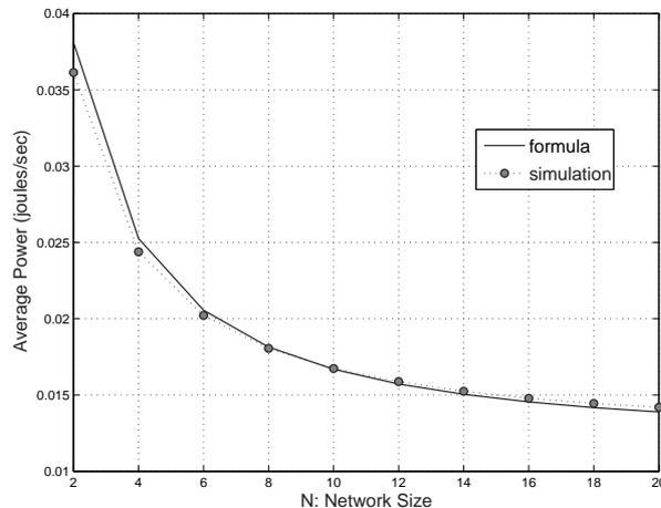
Figure 1.8: Comparison between formula and simulation values for  $\bar{P}$ .
