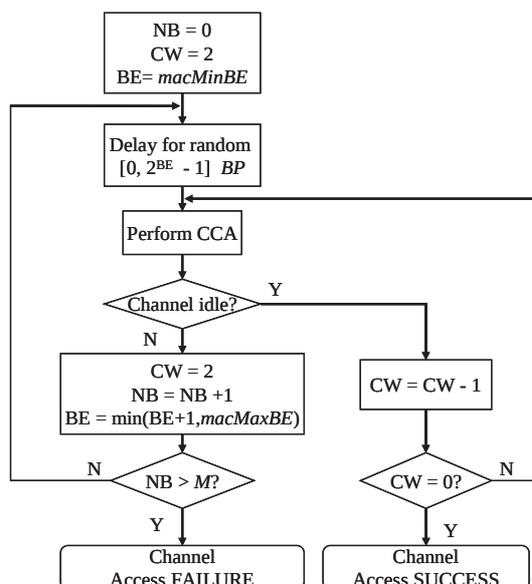
Figure 1.3: Flow chart of the channel access procedure.
