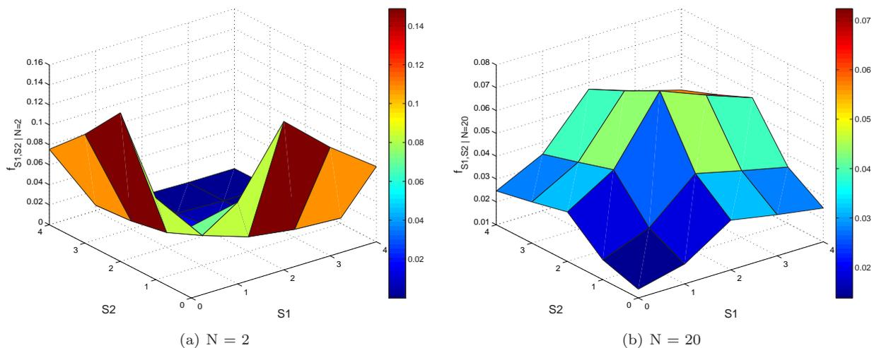
Figure 1.14: Joint pmf of the backoff stages of two nodes  $f_{S_1, S_2 | N}(i, j)$ .
