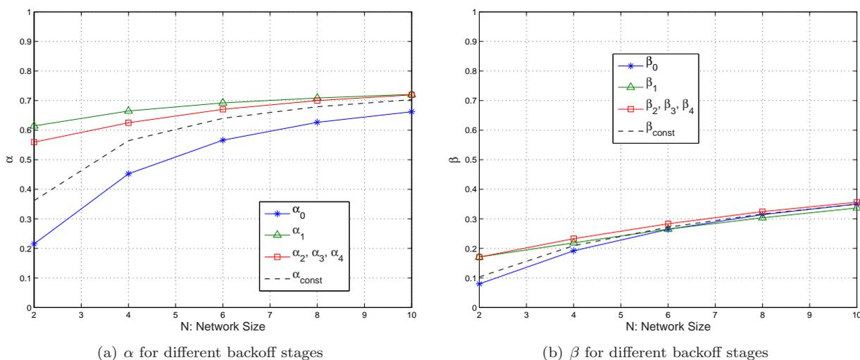
Figure 1.12: Dependence of  $\alpha$  and  $\beta$  on the backoff stage.
