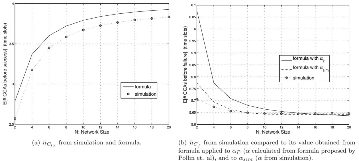
Figure 1.10: Comparison between formula and simulation values for  $\bar{n}_{C_{tx}}$  and  $\bar{n}_{C_f}$ .
