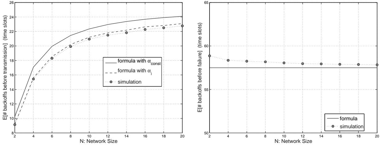
(a)  $\bar{n}_{B_{tx}}$  from simulation compared to its value from formula applied to the constant  $\alpha$ , and to  $\alpha_i$ . (b)  $\bar{n}_{B_f}$  from simulation and formula applied to constant  $\alpha$ .
