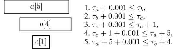
Figure 1: Example event sequence and induced constraints.
