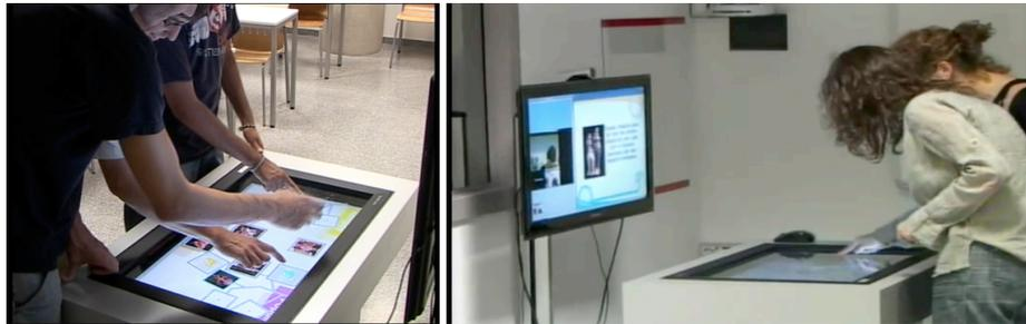
**Fig. 1.** The system includes two remotely located stations. *Right:* Participants interact on a horizontal surface while sharing the same workspace with remote partners. A vertical screen shows a video feed facilitating communication between the two locations. *Left:* Simultaneous co-located participants categorizing objects by country of origin and by functionality.
