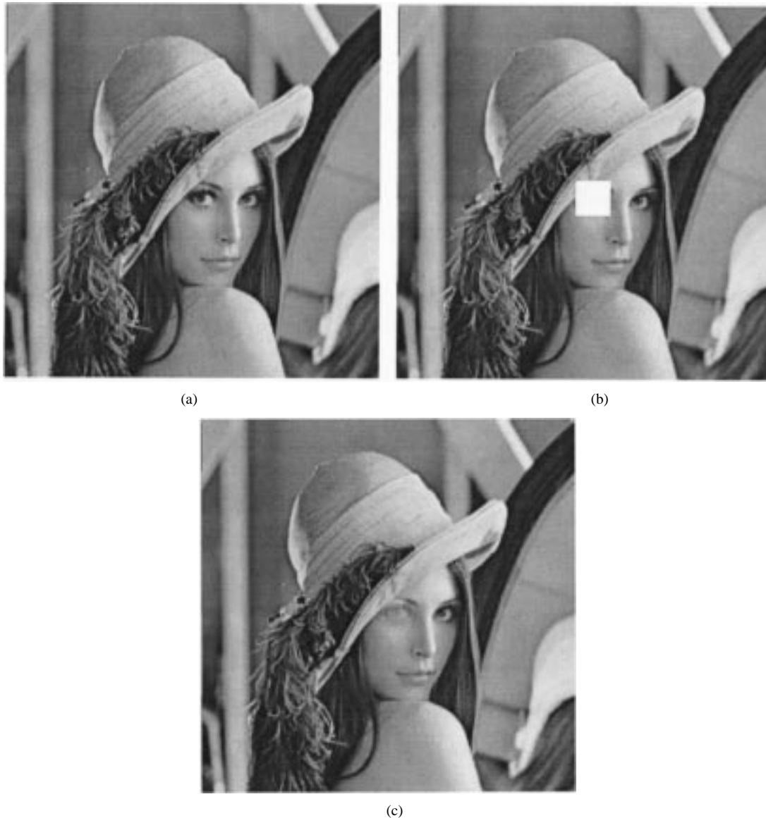
Fig. 4. (a) Original image, (b) original image with missing region, and (c) filled-in image when the gradients inside the white square are known.
