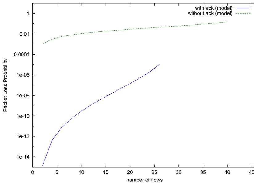
**Fig. 5** The packet loss probability is significantly higher when acknowledgements are suppressed.
