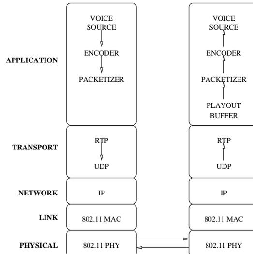
**Fig. 2** The figure presents the complete protocol stack in implementing VoIP over IEEE 802.11.
