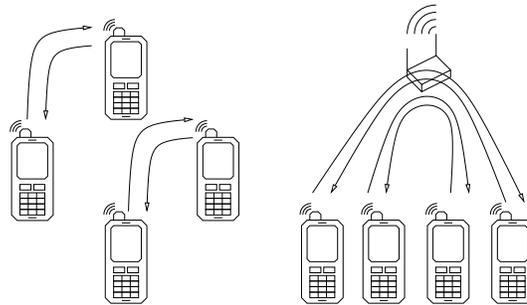
**Fig. 1** This figure compares ad-hoc (left) to infrastructure-based (right) VoIP calls in a IEEE 802.11 network.
