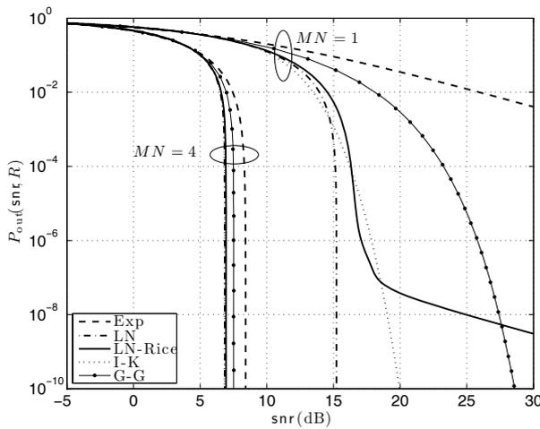
Fig. 3. Outage probability with CSIT for lognormal-Rice (solid), exponential (dashed), lognormal (dot-dashed), I-K scintillation (dotted) and gamma-gamma (solid with markers) with  $B = 1$ ,  $Q = 2$ ,  $R_c = 1/2$ ,  $r = 10$ ,  $\alpha = 2$  and  $\sigma_I^2 = 1$ .
