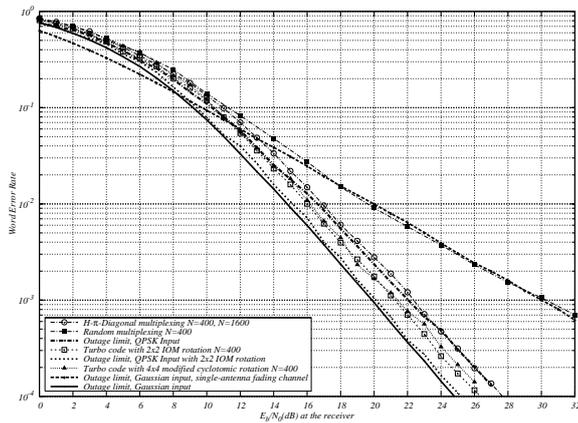
Fig. 2. NAF half-duplex fading channel, turbo code RSC (17, 15)<sub>8</sub>, QPSK.
